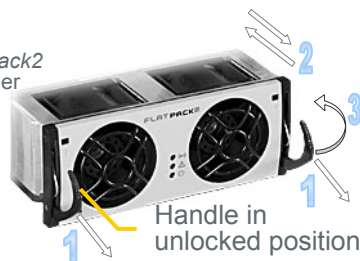
Figure 2 Flatpack2 rectifiers's locking mechanism
