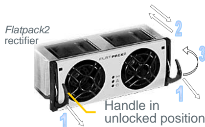
Figure 4 Flatpack2 rectifiers's locking mechanism
