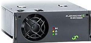
Part number 241115.705. In addition to the High Efficiency feature — refer to chapter "Flatpack2 Rectifier 48V, 2000W HE", page 11 — the rectifier's Wide DC Output Range (WOR) enables support for battery banks of both NiCd and Pb. From the controller, you can configure from 38 to 40 cells in NiCd battery banks, and 24 or 30 cells in Pb battery banks.
