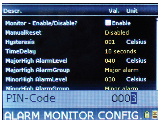
Figure 6 - Enabling Temperature Probe Monitor
