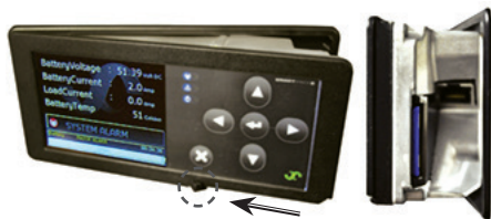
Figure 1 - Smartpack2 Master Controller Display and SD card slot
