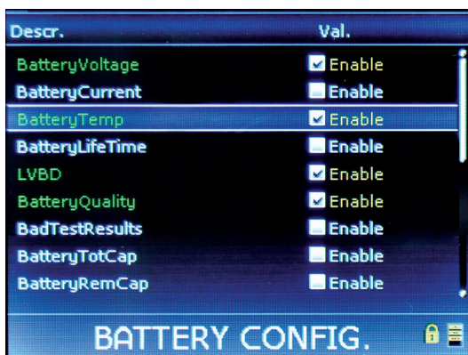
Figure 7 – Enabling Battery Temperature Monitor
