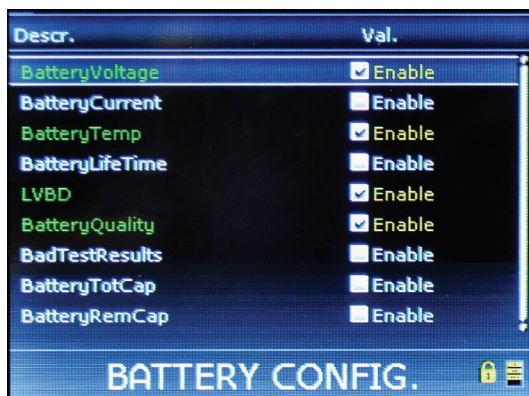
Figure 2 – Enabling Battery Voltage
