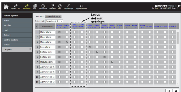
Figure 6 - Alarm Outputs Page (Smartpack R Controller)
