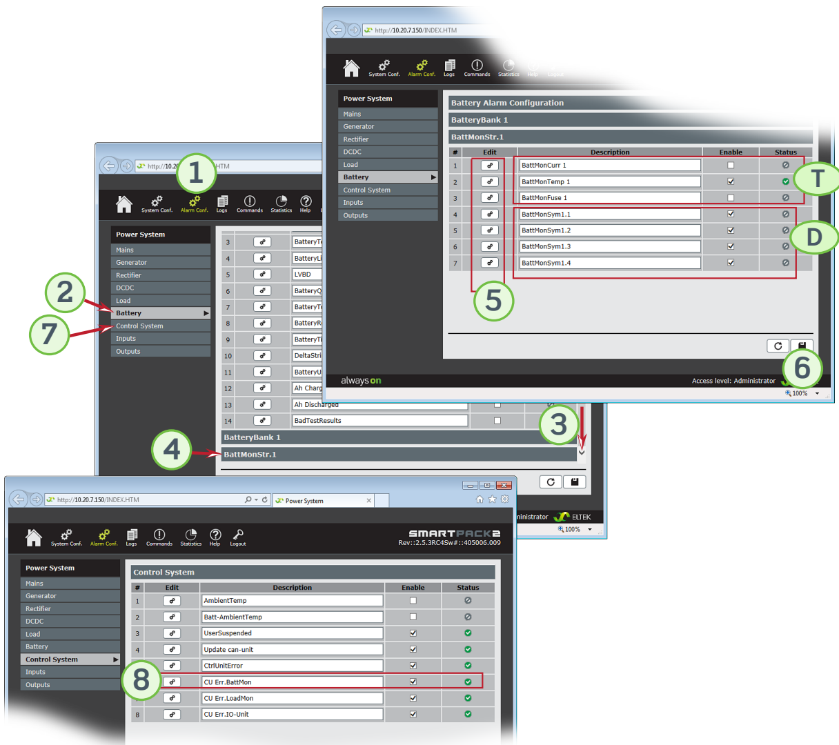
Figure 12. Configuration of the Battery Monitor's inputs via Web browser
