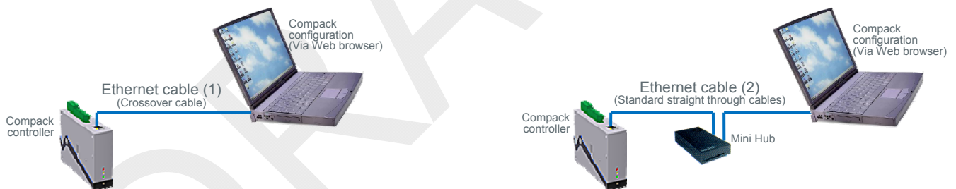
Figure 9 Controller's access from a stand-alone PC using a Ethernet crossover cable or using a standard mini HUB
