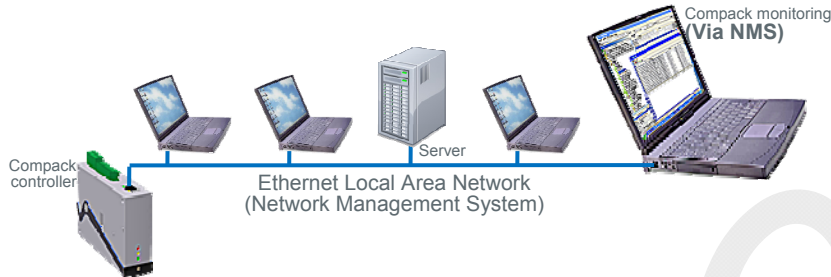
Figure 13 Power system remote monitoring via NMS.
