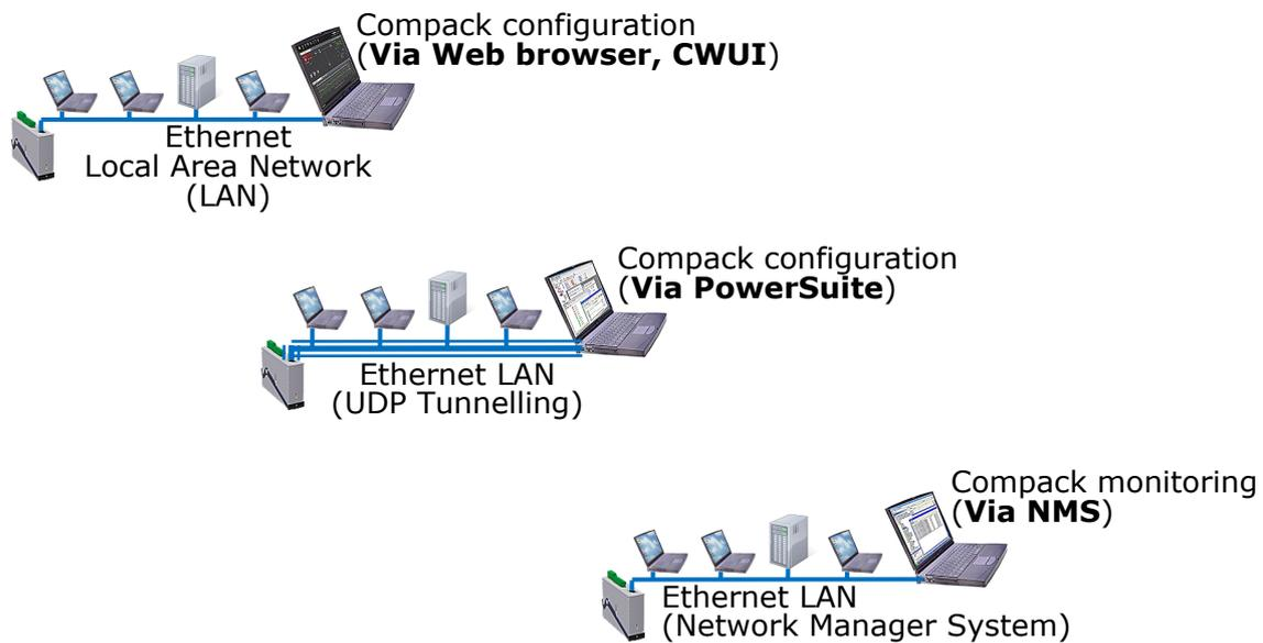
Figure 15 Power system configuration via Web browser, PowerSuite and NMS.
