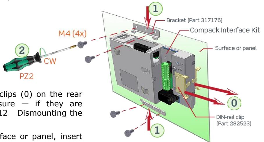
Remove the two DIN rail clips (0) on the rear of the kit's metal enclosure — if they are mounted. Refer to Figure 12 Dismounting the DIN rail clips, page 12
