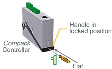
1. **Open the handle** by inserting a screwdriver into the hole to release the spring mechanism
