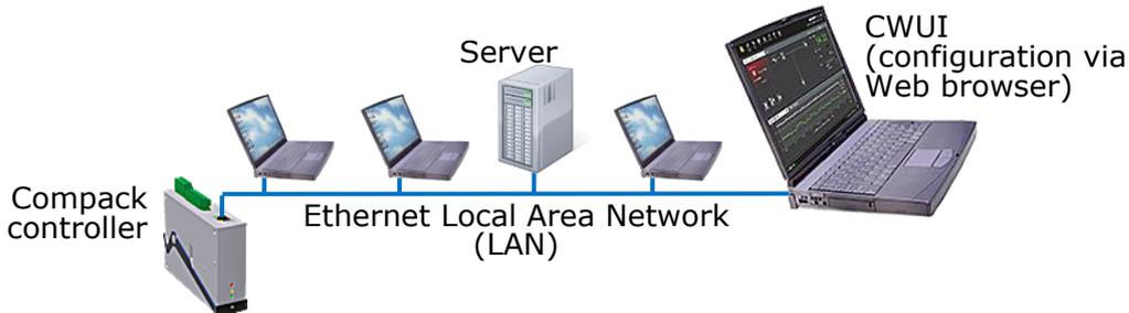
Figure 16 Power system configuration via Web browser.
