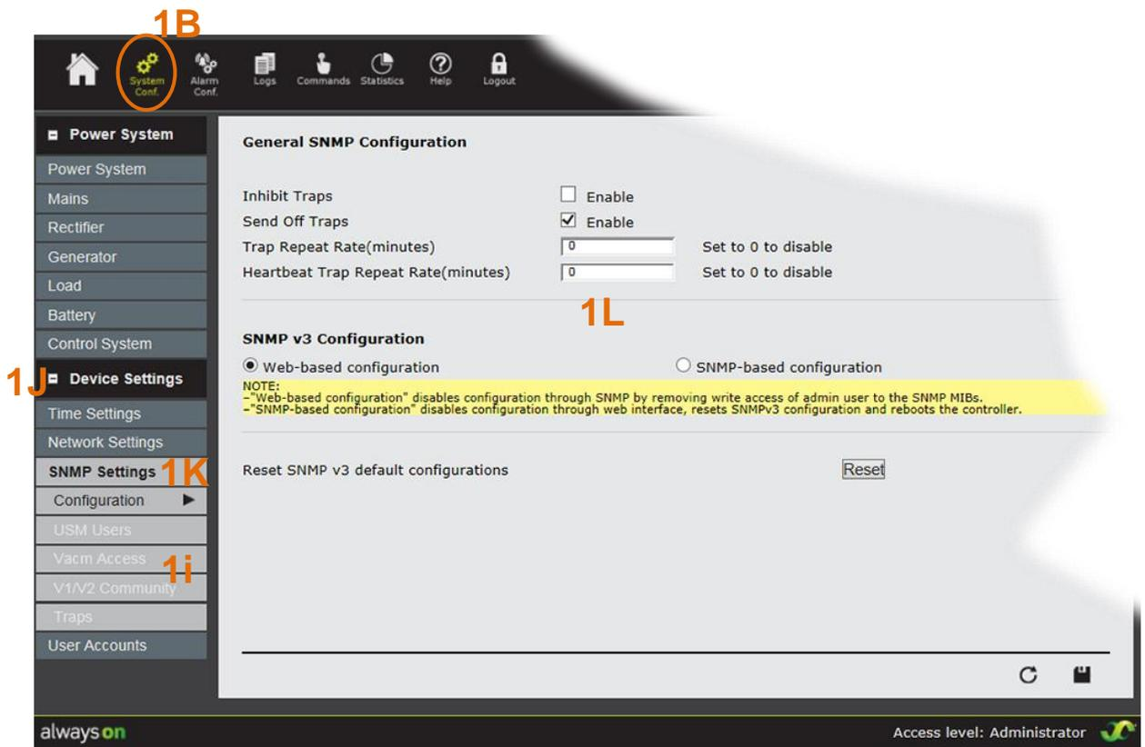
(CWUI interface: example of Compack controller’s configuration pages)
