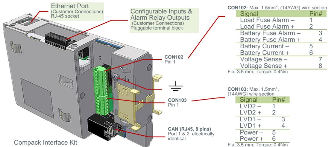
Figure 14 *Compack Interface Kit's* internal system connections (CON102 & CON103)
