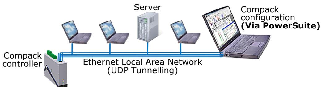
Figure 17 Power system configuration via PowerSuite application.
