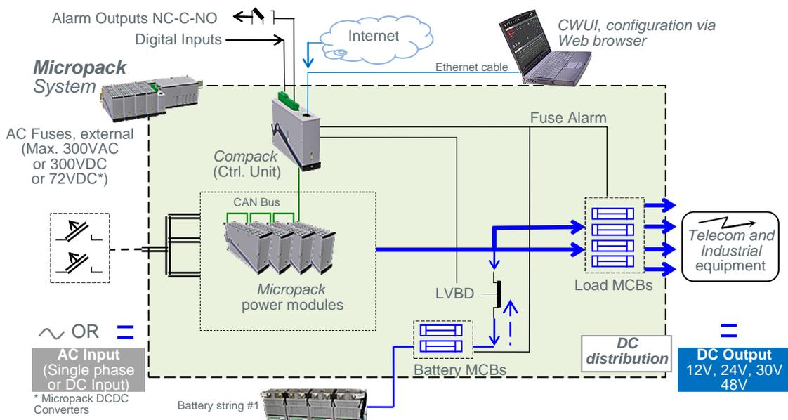
*Figure 1* Example of a typical *Micropack PS* system used as a power supply for telecom and industrial equipment. The system is fed from an external AC mains supply or DC supply, and consists of power modules, a control unit and DC distribution unit with LVBD contactor, all mounted on a DIN rail. External battery bank can be connected.
