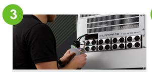
Unplug it. Power modules will run in standalone mode temporary at default voltage.
