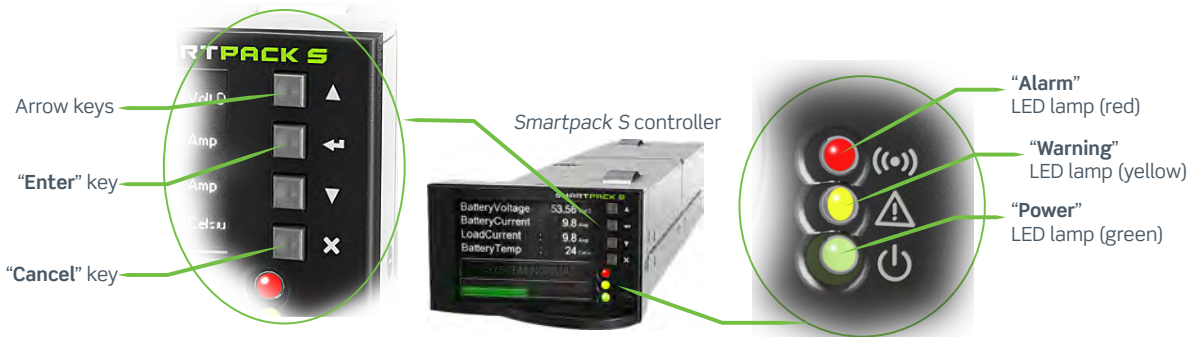
Figure 5. Smartpack S controller's front keys and indicators
