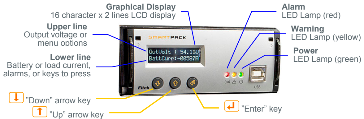
Figure 11 Smartpack controller's front keys and indicators
