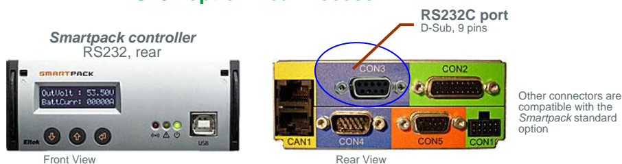
Figure 19 The Smartpack controller, RS232 option, rear. Front and rear connections
