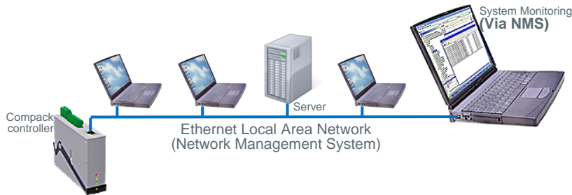
Figure 27 Power system remote monitoring via NMS.
