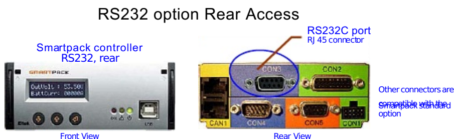
Figure 14 The Smartpack controller, RS232 option, rear. Front and rear connections
