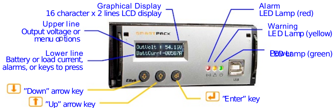
Figure 19 Smartpack controller's front keys and indicators
