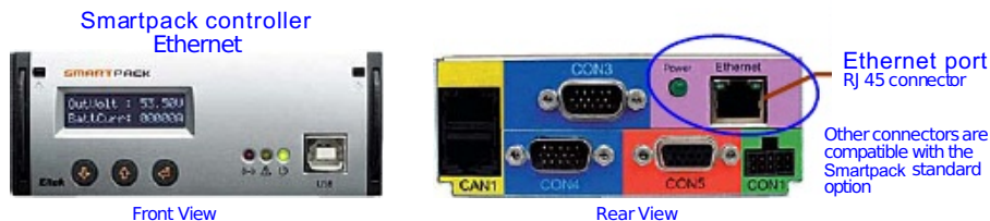
Figure 12 The Smartpack controller, Ethernet option. Front and rear connections
