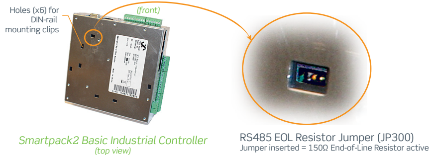
Figure 4. Location of the RS485 EOL resistor jumper in the SP2BI controller
