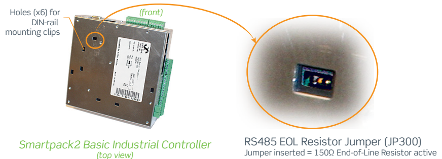
Figure 4. Location of the RS485 EOL resistor jumper in the SP2BI controller
