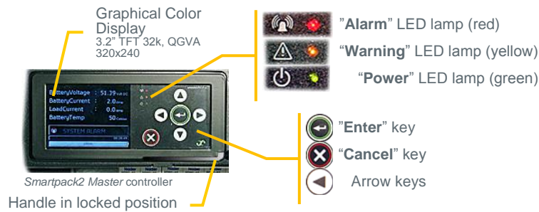
Figure 4 Smartpack2 Master controller's front keys and indicators
