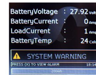
Press key to view Alarms. (ALARM only appears when an alarm is active.)
