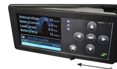
Open the controller by sliding the lever from right to left.
