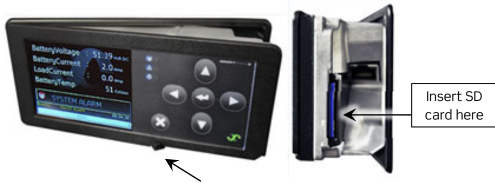
Figure 2 - Inserting the SD Card
