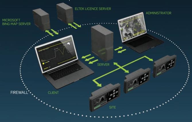
Communication between the server and the on-site controllers takes place within the boundaries of a firewalled environment.
