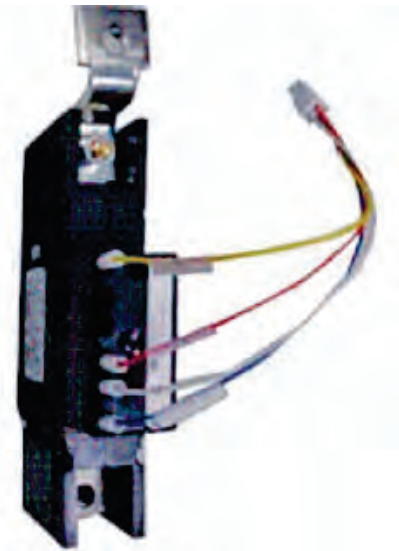
Figure 21 – GJ Breaker Assembly
