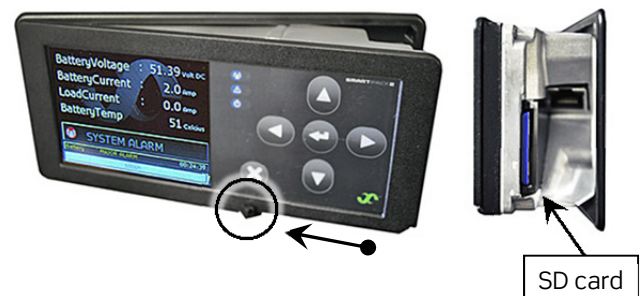
Figure 7 - Controller SD Card
