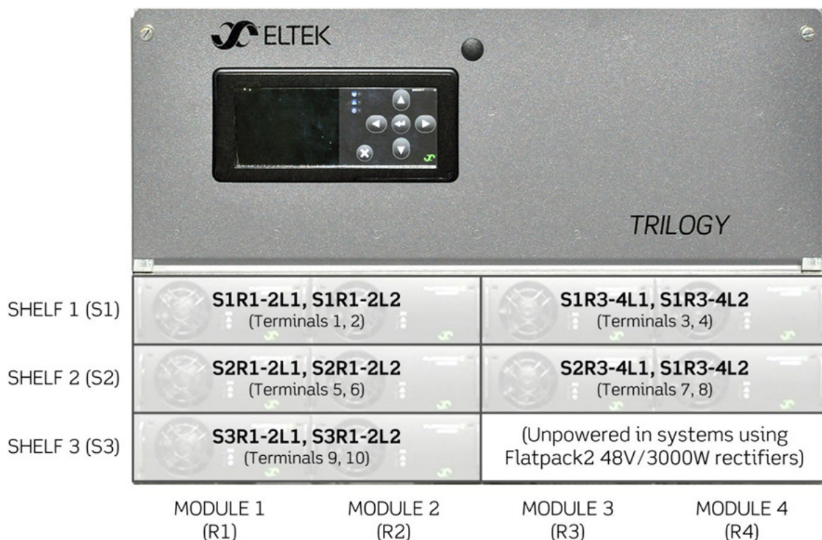
Figure 19 - Terminal Block Assignments, Dual-Feed
