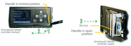
Open the controller by pushing the handle toward you with your finger or pen. Connecting the LAN cable via RJ-45 socket into the controller.
